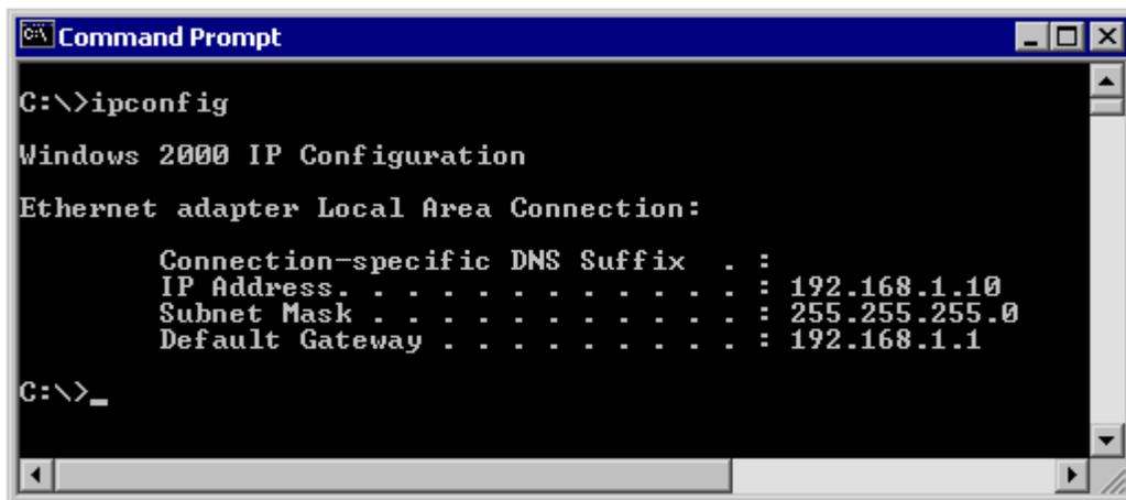
This first screen shows the IP address, subnet mask, and default gateway. The IP address and the default gateway should be in the same network or subnet, otherwise this host would not be able to communicate outside the network. In the figure the subnet mask tells us that the first three octets must be the same to be in the same network.
