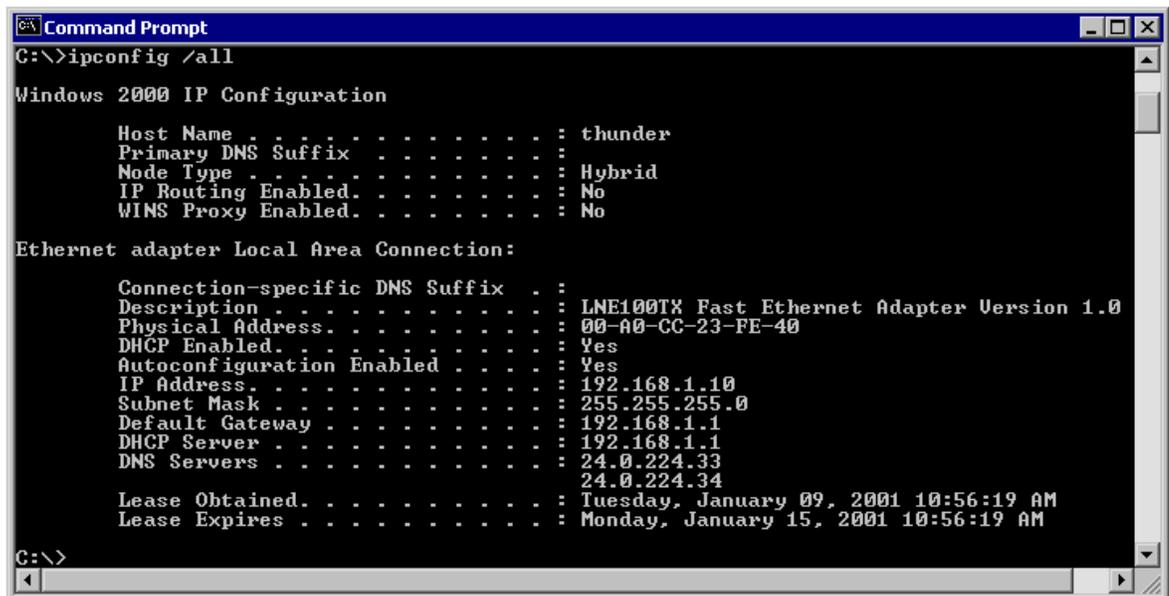
The host name, including the computer name and NetBIOS name should be displayed. Also, the DHCP server address, if used, and the date the IP lease starts and ends should be displayed. Look over the information. Entries for the DNS, used in name resolution servers, may also be present.
